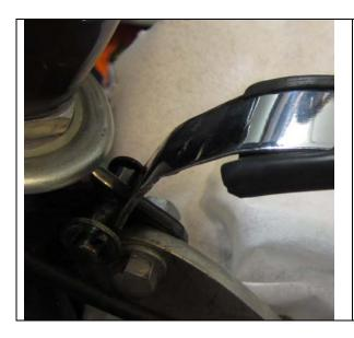
The front mounting of the centre strap is easy enough- just a pin through the front loop of the strap and a frame bracket secured by split pins.
